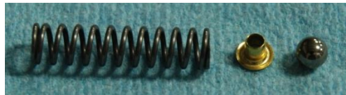
Figure 14, Return Line Back-Pressure Circuit Ball and Spring
