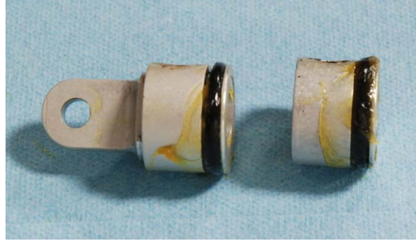
End plugs with Parker O-Lube and new O-rings installed
