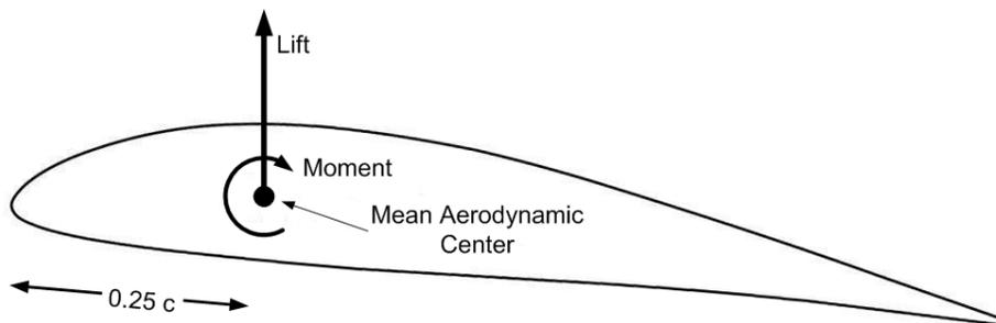
Figure 1, Mean Aerodynamic Center of an Airfoil
