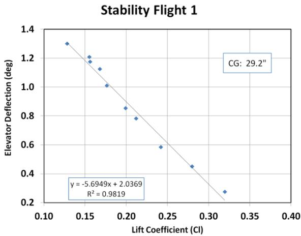
Figure 6, Stability Test, Forward CG
