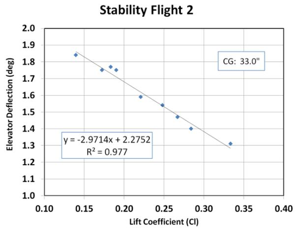
Figure 7, Stability Test, Aft CG
