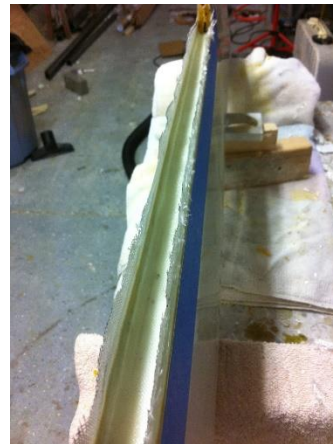
Figure 10, Rear Spar Close-out
