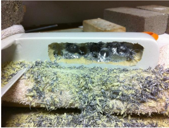
Figure 19, Lead Counter Weight Removal
