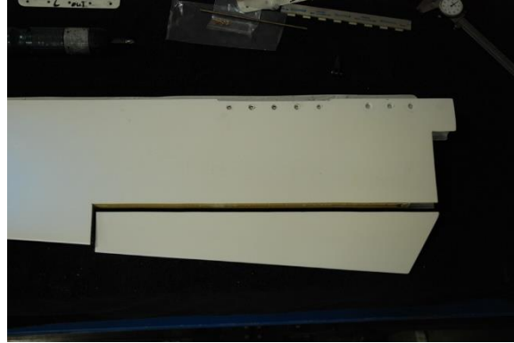
Figure 8, Trim Tab cut from Elevator
