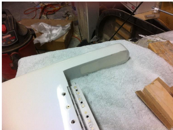
Figure 21, Micro Finish of Mass Balance Arm
