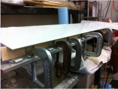
Figure 11, Elevator Hinge Mounting Surface Preparation
