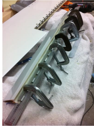
Figure 12, Tab Hinge Mounting Surface Preparation
