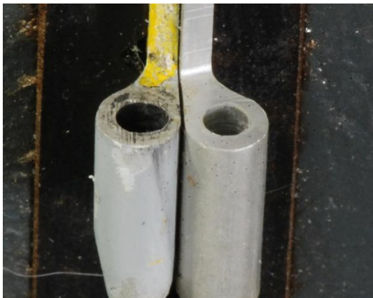
Figure 5, Wear on removed hinge
