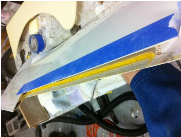
Figure 9, Core material removal
