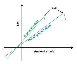
Figure 3, Critical AoA Change in Ground Effect, from NTSB report on G-650 accident
