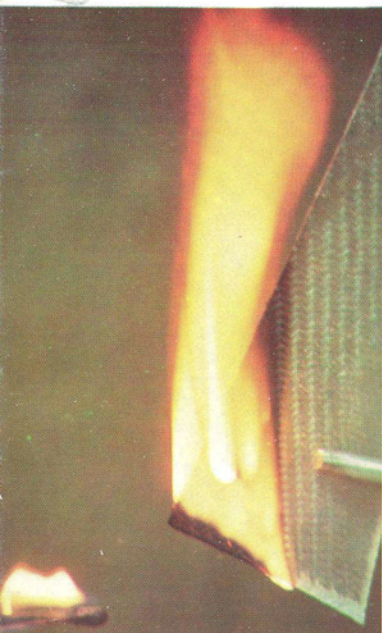
Typical vinylester laminate as used on many kit planes is extremely flammable.
