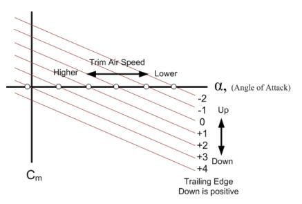
Figure 5, Effect of Elevator Deflection on Trim Speed
