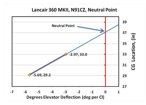
Figure 8, Neutral Point Result by Flight Test
