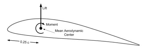
Figure 1, Mean Aerodynamic Center of an Airfoil
