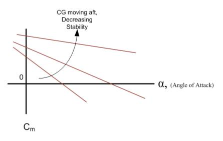
Figure 4, Pitching Moment Slope and Stability
