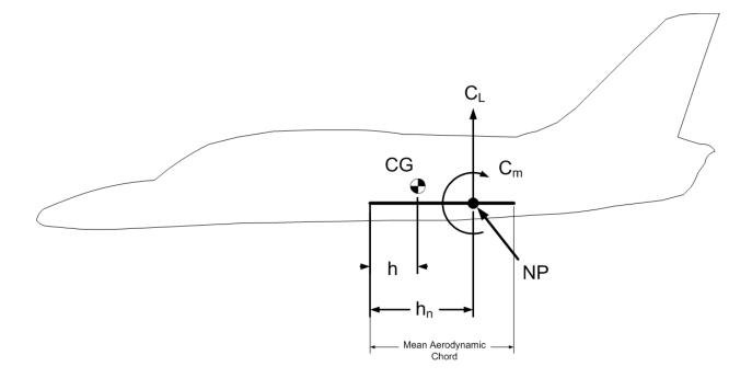
Figure 2, Total Lift and Moment acting on aircraft
