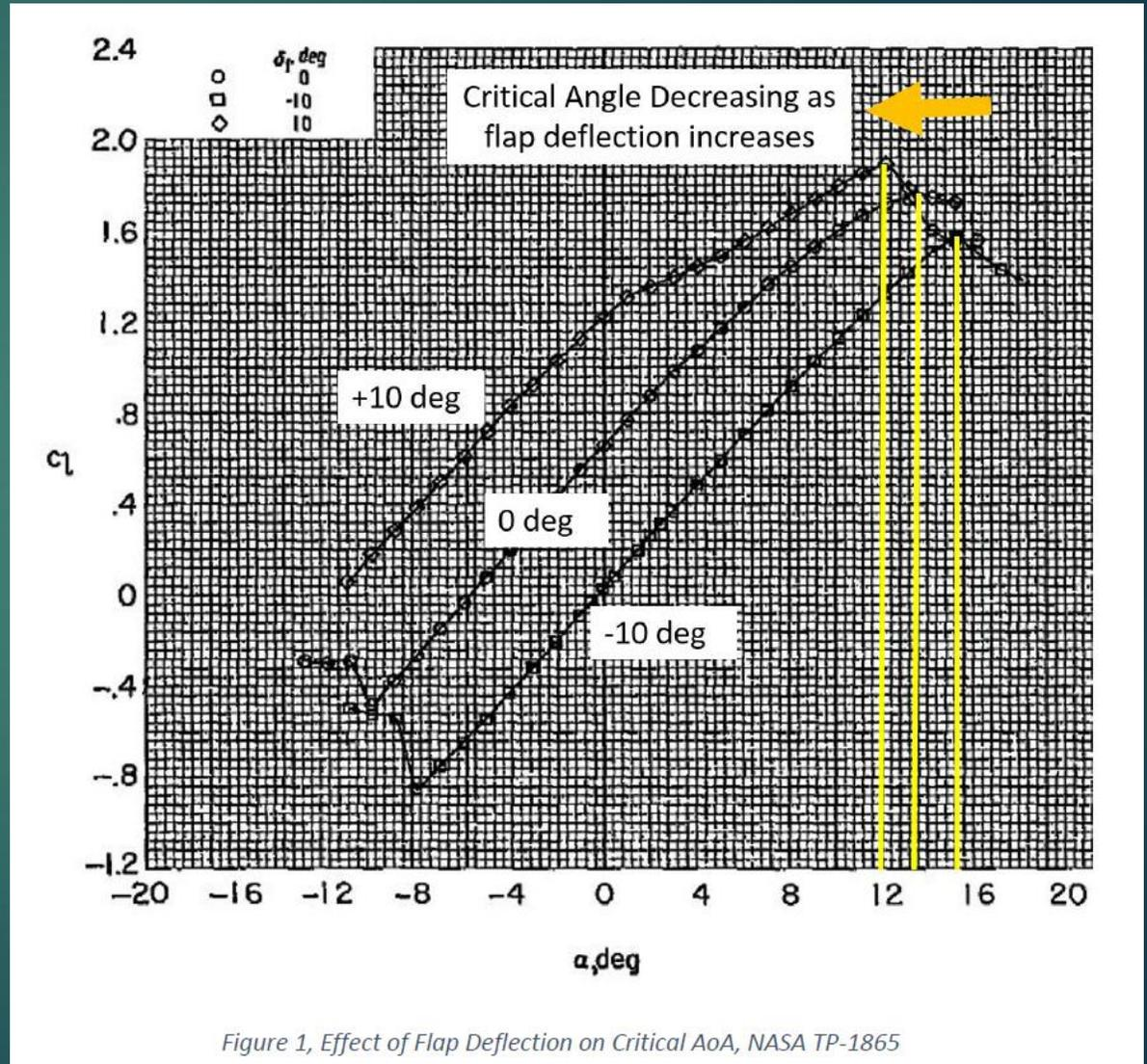
Figure 1, Effect of Flap Deflection on Critical AoA, NASA TP-1865
