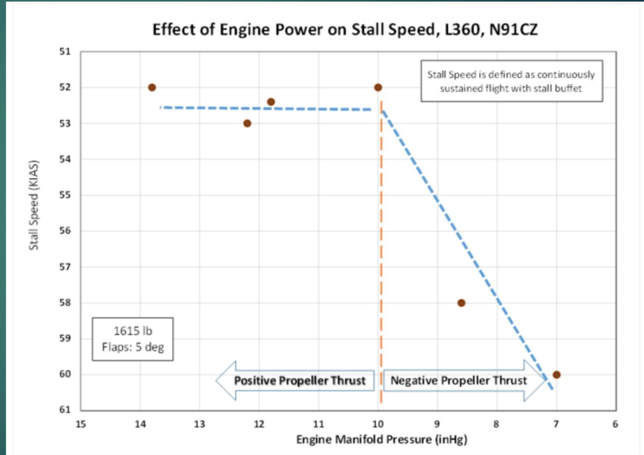
Figure 5, Effect of Propeller Thrust on Stall Speed
