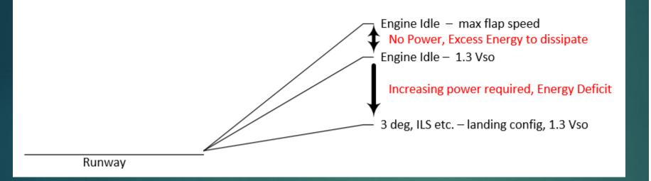
• Excess energy (altitude) can be dissipated by raising the airspeed from 1.3 Vso up to max flap extension speed
