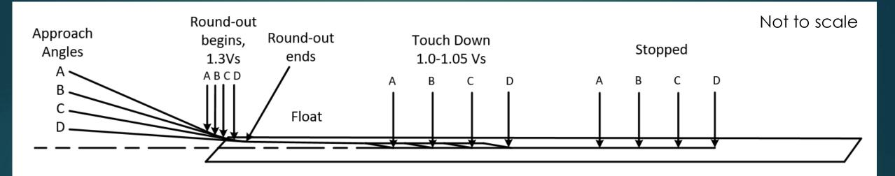
If the round out could be flown with perfect precision and repeatability, the steeper the approach, the shorter the landing. Due to:
