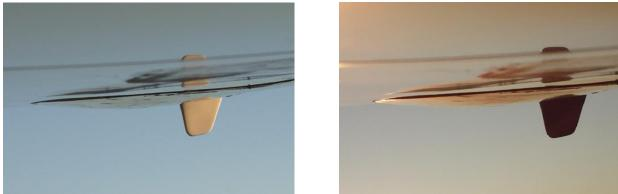
Figure 6, New Carbon Doors In-flight
